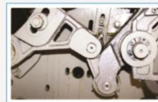
The 6 Connecting Rod Weft Insertion Mechanism
